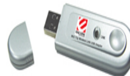
TARJETA DE RED ENCORE WIRELESS USB 802.11G 54 MBPS
